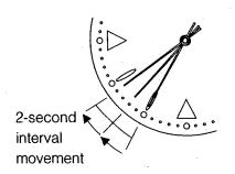
When the second hand is moving at 2-second intervals (moves two gradations at a time every 2 seconds), this indicates that the watch is insufficiently charged. Although the watch continues to run normally at this time, if roughly 11 days elapse after 2-second internal movement has begun, the watch stops running. When this happens, charge the watch by wearing it on your wrist until it returns to normal 1-second internal movement.
