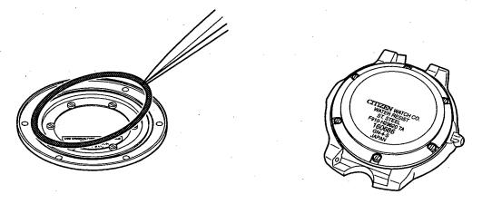
Note: Tighten the six case back screws in the diagonal order. At this time, fit the washers to them without fail.
