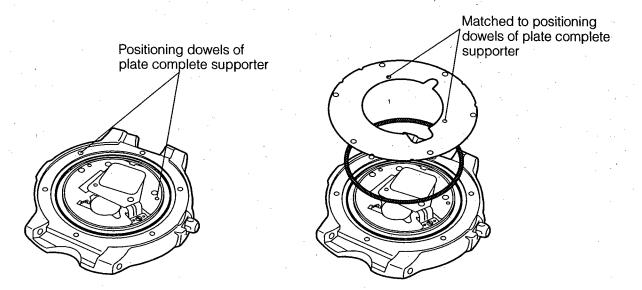
4. Fit the packing to the case back, then set the case back and tighten the case back screws. Set the case back so that the stamp on it will be in parallel with the crown.
