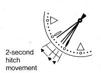
Although the watch hands begin to move when the watch has been recharged after it has stopped as a result of being insufficiently charged, since the time is incorrect, the second hand moves in a 2-second hitch movement (moves irregularly once every 2 seconds) indicating that the time is incorrect.
